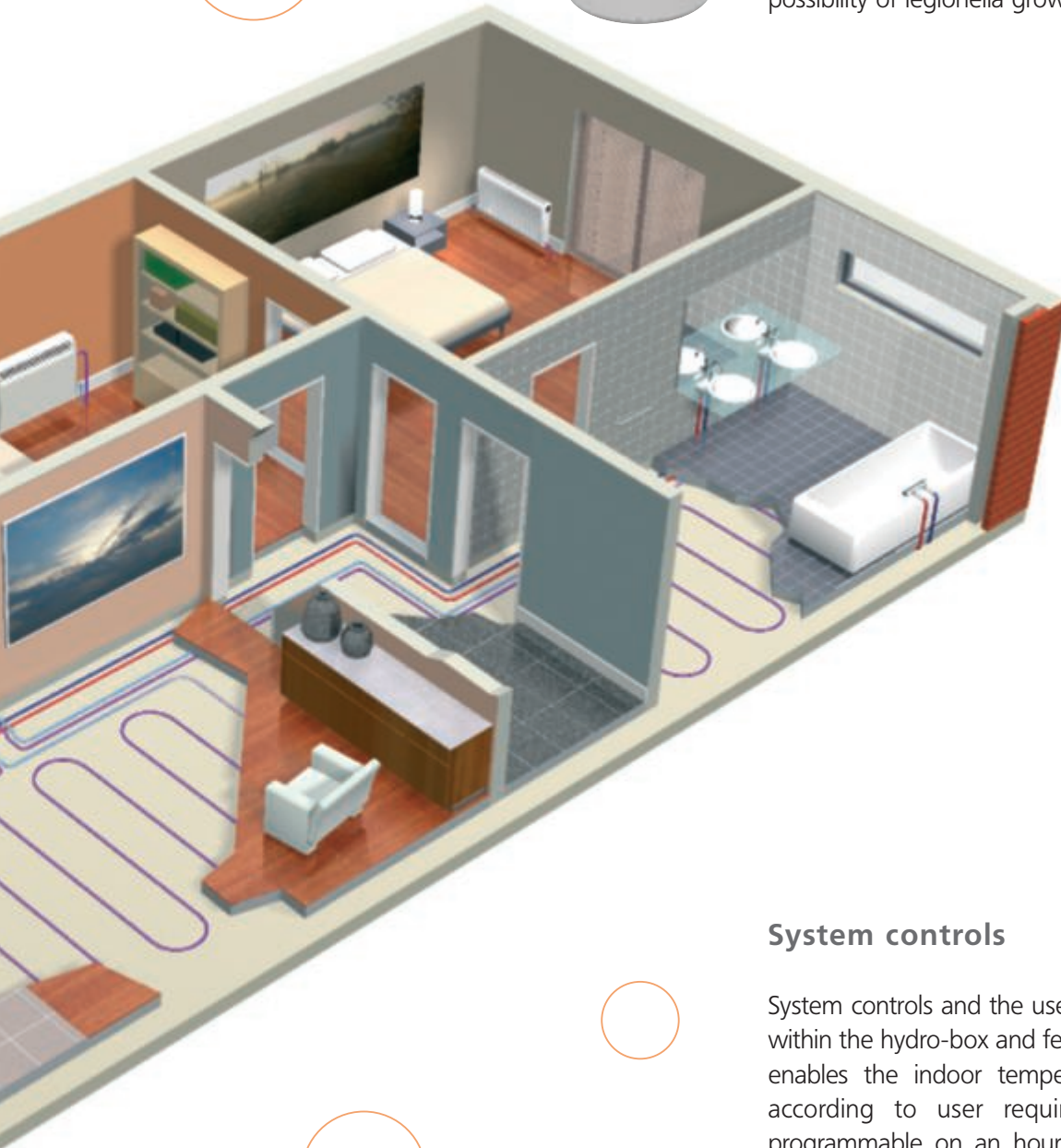
Typical system configuration including optional sanitary hot water tank and optional cooling
